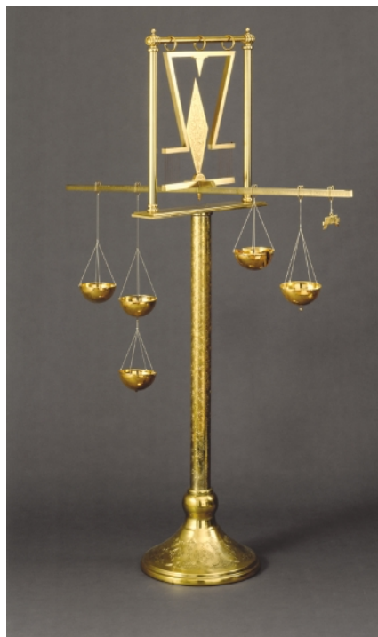
This extremely exact ‘Balance of Wisdom’ was built at the Institute for the History of Arab–Islamic Sciences according to the description by Abdarrahmānal-Khāzini from Khorasan in Northeast Persia, who perfected and described it in the first half of the twelfth century. Image courtesy of Fuat Sezgin, Institute for the History of Arab–Islamic Sciences, University of Frankfurt, Germany.
